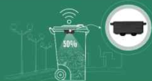
Bin-level sensors (ultrasonic or weight-based) for fill monitoring
